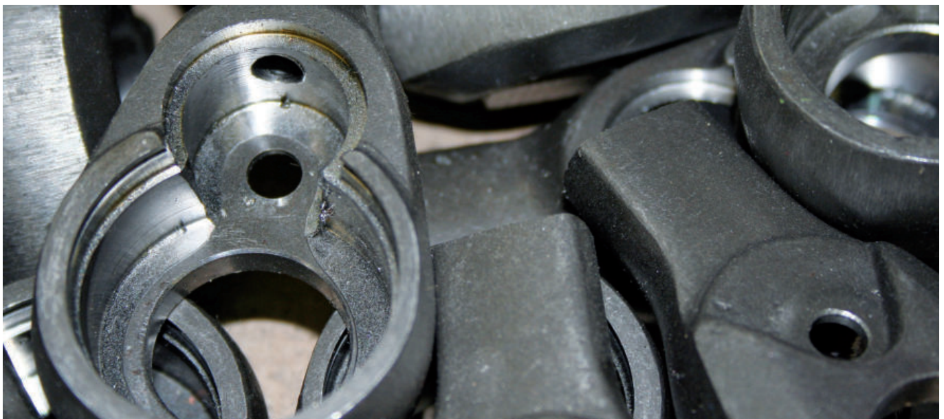
Rohlinge (Ratschenkopf) blanks (ratched head)
