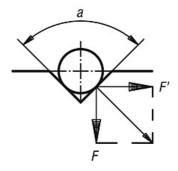
$a = 60^{\circ}$ ,  $F' = 1.732 \times F$   $a = 90^{\circ}$ , F' = F $a = 120^{\circ}$ ,  $F' = 0.577 \times F$
