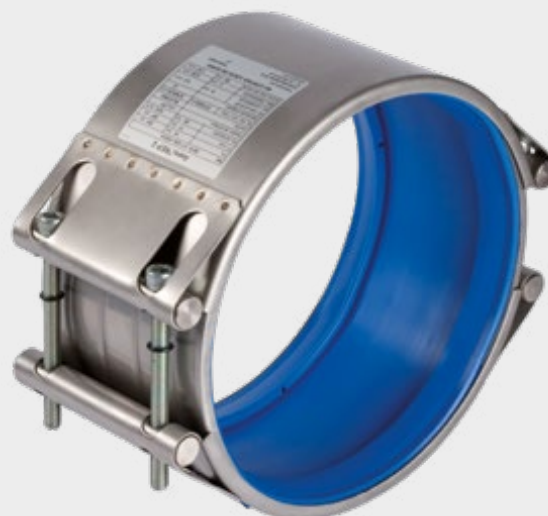
Blue silicone seal Suitable for drinking water and industrial water. Temperature range from -55^{\circ}\text{C} to +200^{\circ}\text{C}
