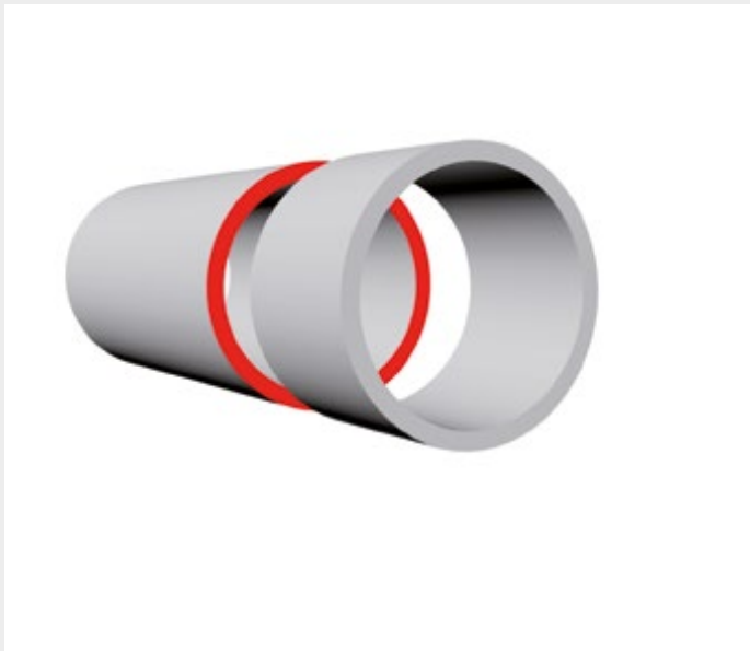
Connection of pipes with a gap between the pipe ends
