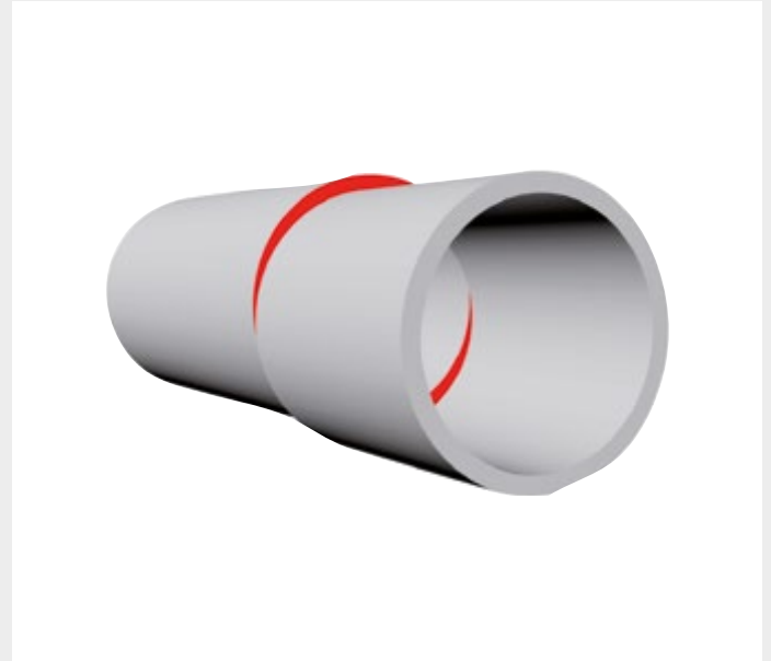
Connection of pipes with an offset
